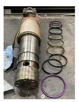
Seal failures will manifest as an external oil leak, which can be misidentified as a motor case seal failure or compromised shear function, such as low power, difficulty opening the jaw, or a steady jaw drift. These can typically be troubleshot with hydraulic gauges or a manifold bypass test.
