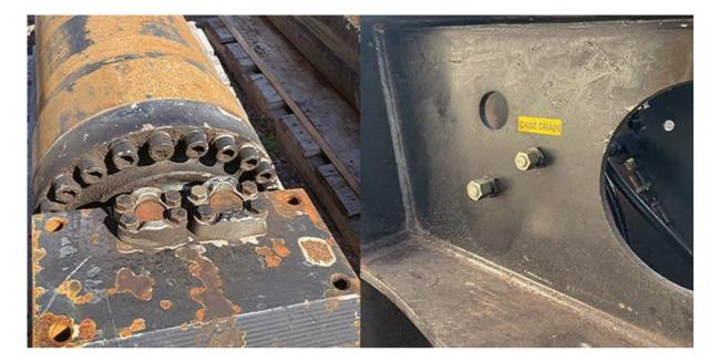
Cylinders, swivels and rotation components can also be ruined if an attachment is not prepped for storage. In warm weather, the oil in the components will heat up, expand and push out, contaminating everything around them. So not only can the expensive components be ruined, but the base carrier gets contaminated and damaged as well.
