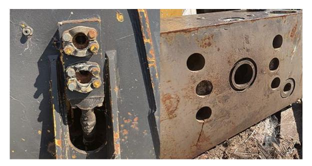
The Code 62 ports in the cylinder must be capped with correctly sized plugs that contain O-rings. O-ring face seal rotation bulkheads must be plugged with the correct face seal caps. Failure to do so will result in moisture and dirt entering the system, causing contamination and corrosion that can result in the wear, faulty operation and rust pitting of finely machined, tight tolerance parts.
