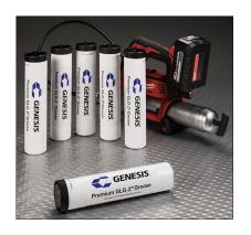
Just as important as the interval, is using the right type of grease! Our recommended grease intervals are 4 and 8 hours, and we recommend GLG-2® extreme pressure lithium grease, P/N 6302601. Using cheap lubricants or base compounds containing Moly doesn't get the job done.
