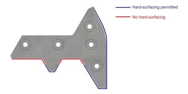
Hard-surfacing in the red areas can lead to premature tooth failure.
