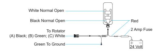
The rotator requires an additional hydraulic circuit. One of the several available options has been supplied with the attachment. These diagrams show the installation of the additional circuit. Refer to the Hydraulic/Rotation Maintenance section of this manual for valve descriptions, functions and settings.
