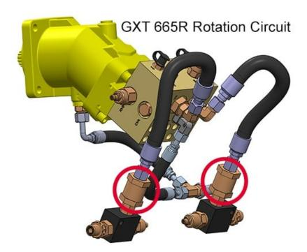
The filters are mounted in the flow control manifold just inside the head where the excavator rotate jump lines are connected. When there is any type of rotation failure, the filters must be changed, and the other circuit components flushed out.
