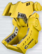
GRS REBAR SHEAR PG 13
